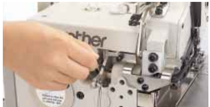
Adjusting upper feed vertical amount
